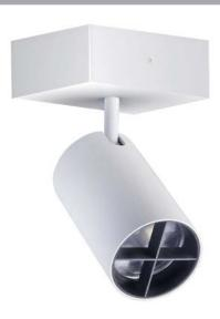
MiniMax LED O-OBM is an accent light designed for mounting on a 4" octagonal outlet box (by others). Luminaire is powered by one of a number of Xicato LED modules – including Artist Series, Designer Series and Vibrant Series modules - all of which are distinguished by extraordinary color consistency (within 1x2-step MacAdam ellipse). See tables below for wattages and efficacies.
