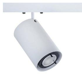
MidiMax NSP is a track mounted 10° or 24° spotlight powered by one of a number of Xicato XTM 9mm modules - including Artist Series and Vibrant Series modules – all of which are distinguished by extraordinary color consistency (within 1x2-step MacAdam ellipse). See tables on the reverse for wattages and efficacies.
