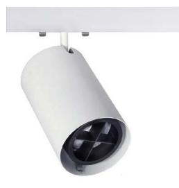
MidiMax Mood Master O is a track mounted accent light equipped with a Lumenetix® Araya® CTM1C 22 mm Color Tuning LED module that produces 90+CRI white light (within 2-step MacAdam ellipse). LED module light output is 1250 lumens drawing 25 input watts maximum.
