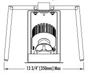
Luminaire is listed for Damp Location, RoHA compliant and prewired with a thermal protector. Removal of the reflector allows access to the LED array, driver and junction box.
